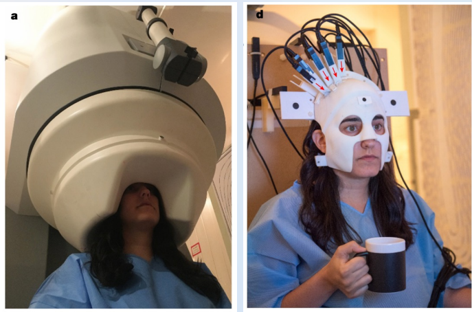
Comparison of SQUID (left) and OPM (right) based MEG in 2018, from 93
